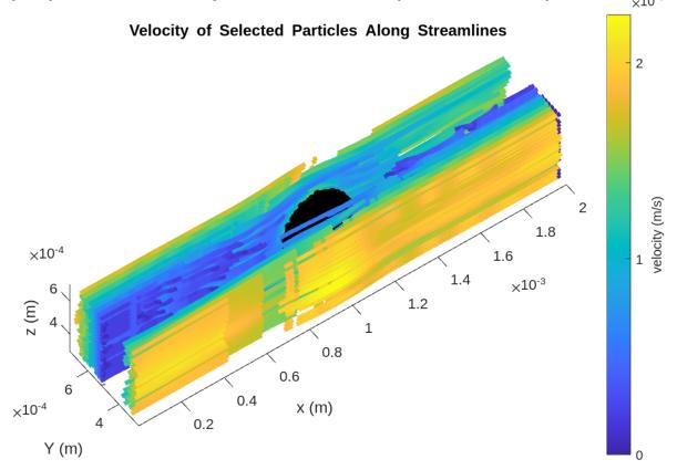
Summary: Step 15 combines numerical data processing (Lagrangian description) with visualization techniques to create a graphical representation of the selected particles' movement (trajectories matching streamlines at the steady state). This plot can be an essential tool for understanding and analyzing the turbulence deveopping in the wake flow.
